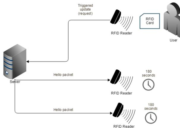
Figure 6. Flow between RFID readers and server
